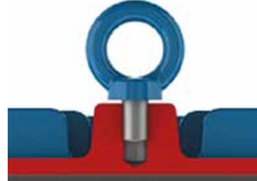
Figure 4.2 - Incorrect tightening of the eyebolt
