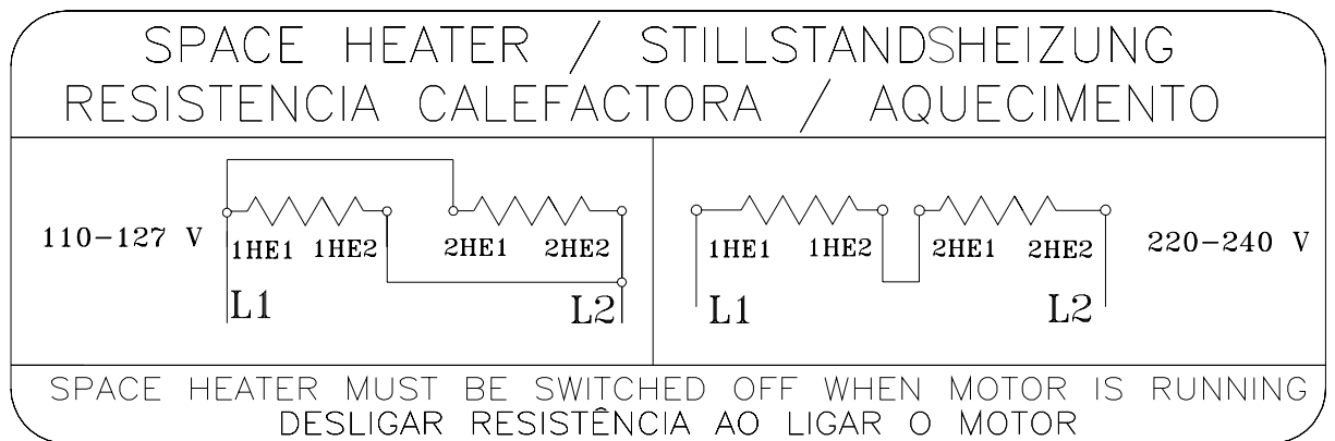
Figure 6.17 - Dual voltage space heater connection
