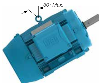
Figure 4.3 - Maximum allowed angle-of-inclination for motor with one eyebolt
