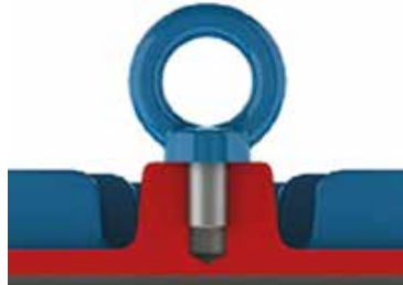
Figure 4.1 - Correct tightening of the eyebolt
