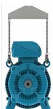
Figure 4.6 - Use of a spreader bar for lifting
